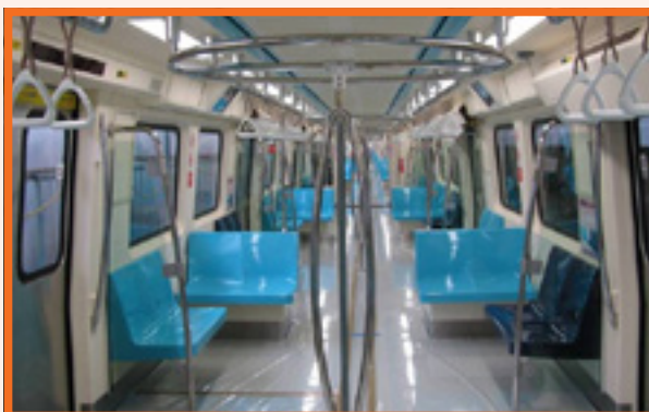
Ring handrails and tri-vertical poles
