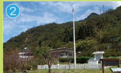
2 Meteorological Observatory The observatory collects and monitors the meteorological data around the reservoir, such as wind velocity, wind direction, atmospheric pressure, solar radiation, evaporation, relative humidity, and temperature. The system is operated by solar power and transmitted by radio to the reservoir operations center, which serves data as basic reservoir operation.
