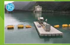
16 Water Quality Vertical Profile Monitoring Station This station is collecting data of water quality from several important parameters, including turbidity, dissolved oxygen, pH, suspended solids, electrical conductivity, water temperature and chlorophyll, to monitor continuously the water quality from surface to bottom, by steps of 5 to 10m.
