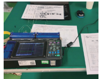
Data logger (surface temperature of magnetic lock)
