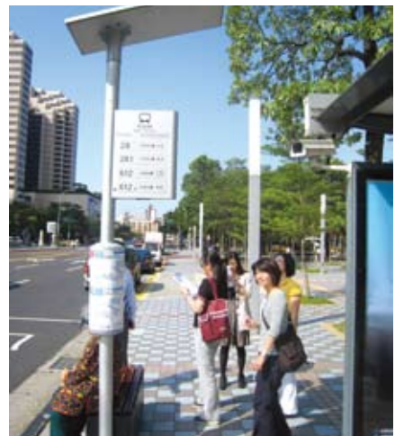
Solar energy stand-alone bus stop signs of the e-Bus system.
