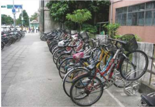
Height-differentiated bicycle stand (neat and space-saving)
