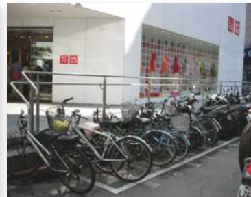
Marked-bicycle parking area (suited for places with relatively high use and roads)
