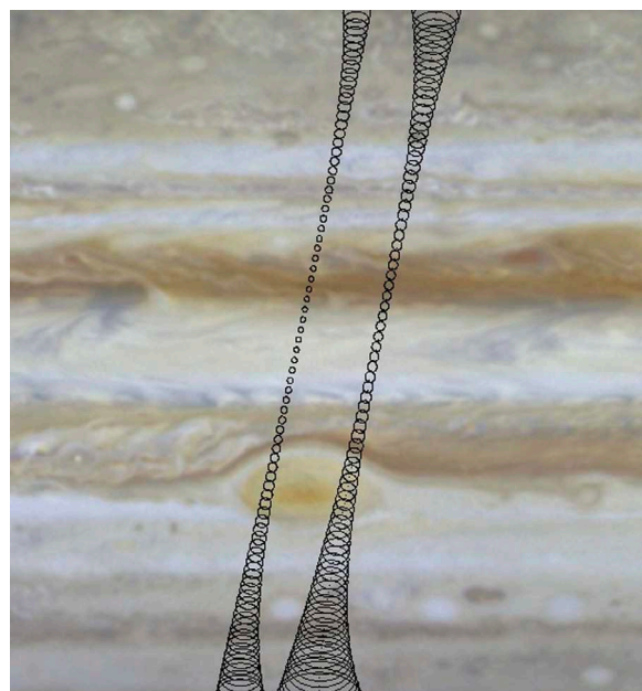
Figure 3. Schematic showing nadir fields of view of the MWR's longest-wavelength channel with its 10^\circ – diameter footprints through a typical Jupiter orbit. Figure courtesy of M. Janssen, MWR PI
