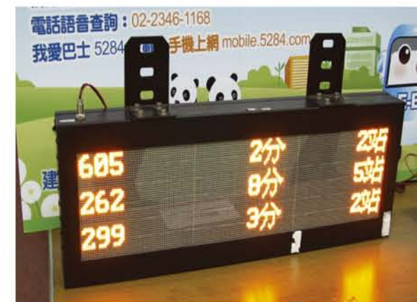
LED式智慧型公車站牌 LED module used in the smart bus stop signs
