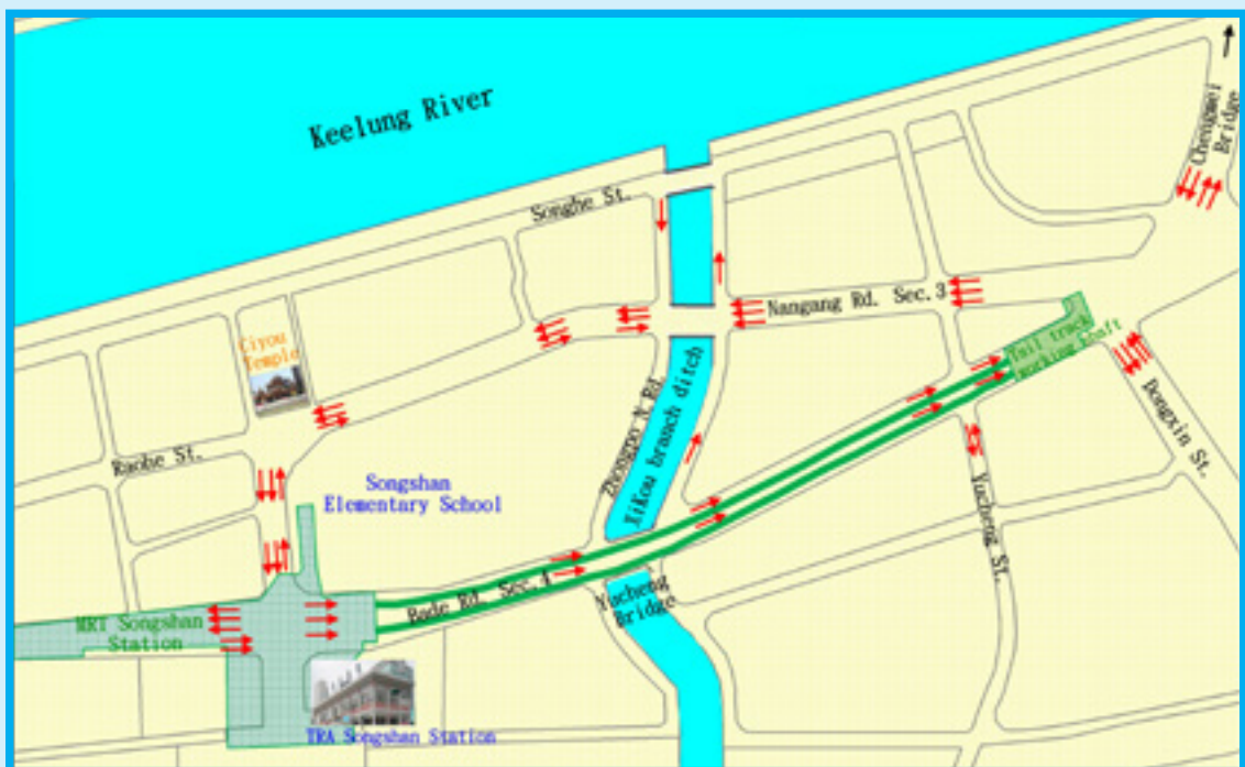
Traffic maintenance layout for Yucheng Bridge reconstruction and tail track construction
