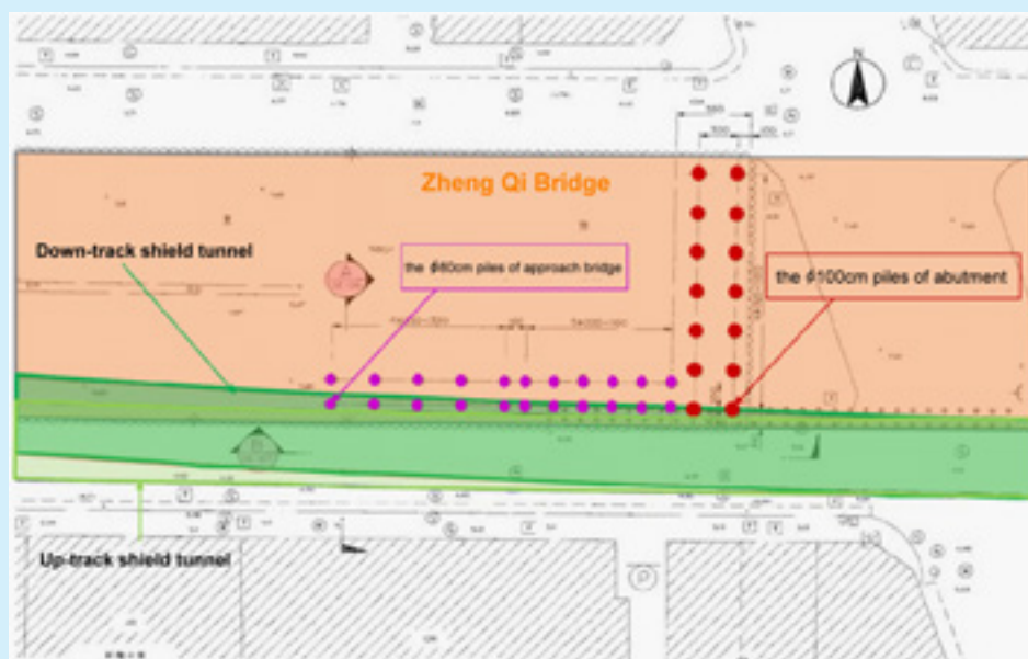
Remaining foundation piles belonging to Zhengqi Bridge
