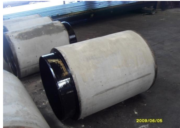
Fig.16 short segment pipe with cement coating
