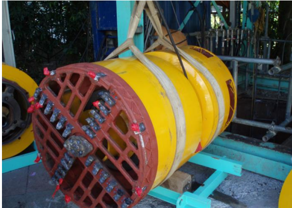
Fig.15 boring auger machine for pipe jacking
