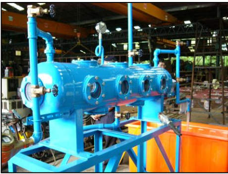
Fig. 3-1 Pipe-Form Emergency Storage Tank
